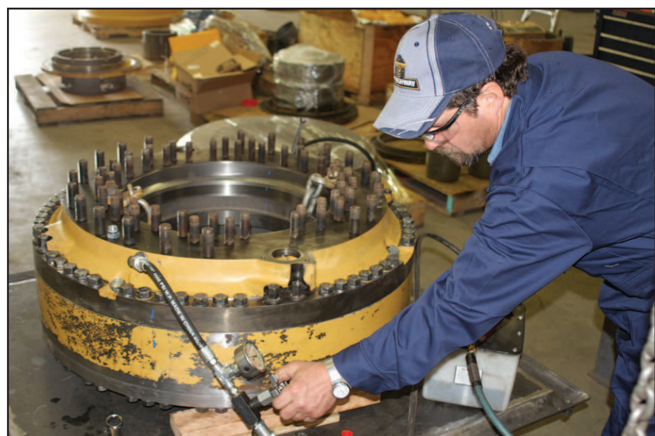
Mark Troumbly testing a CAT Brake that was rebuilt in the Ellefson Off Highway Shop.
