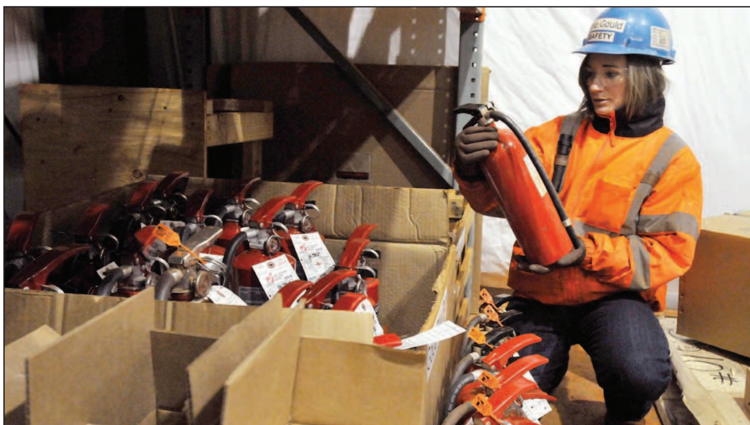
Gina Gould checks pressure gauges on fire extinguishers.
