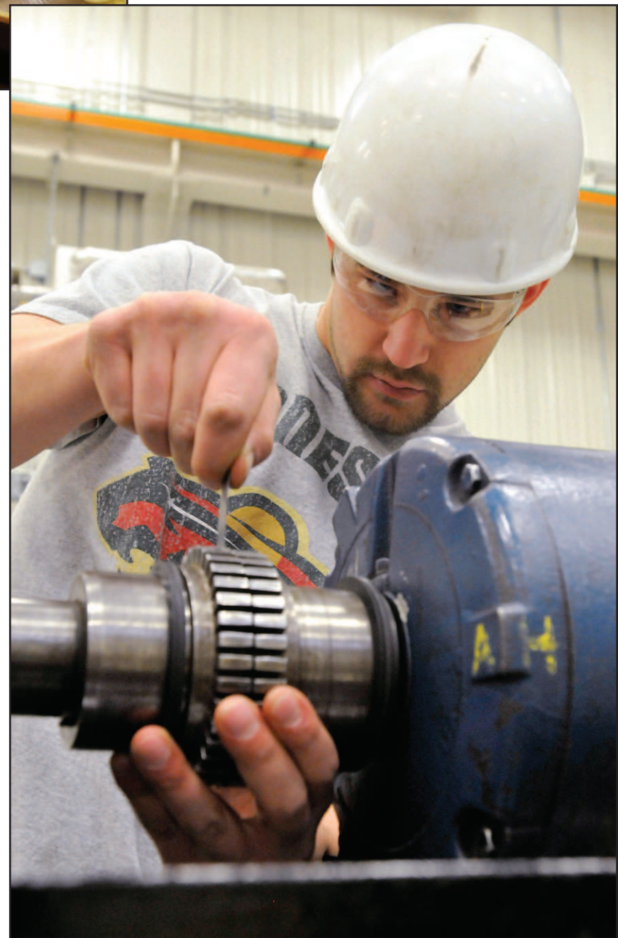
Jack Stavenger adjusts and repairs an electric motor.
