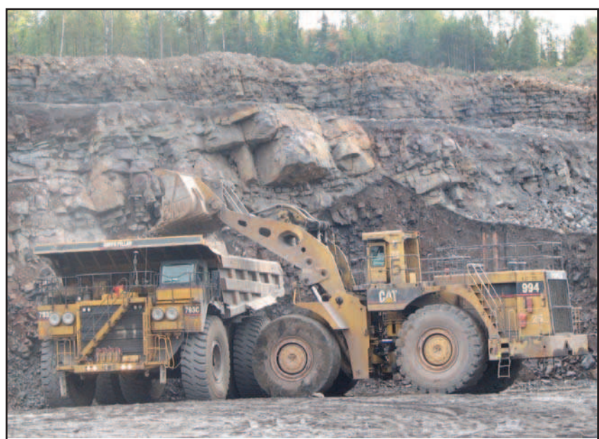
Blasted rock is loaded into a truck to be carried to the crusher.
