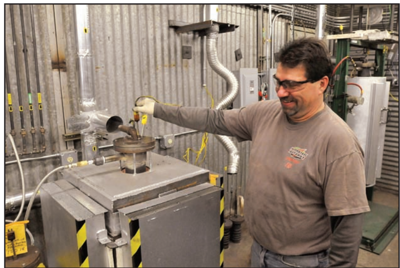
Pat Casey adjusts a test furnace. The furnace can be fired with different fuel mixtures to simulate mine operations.
