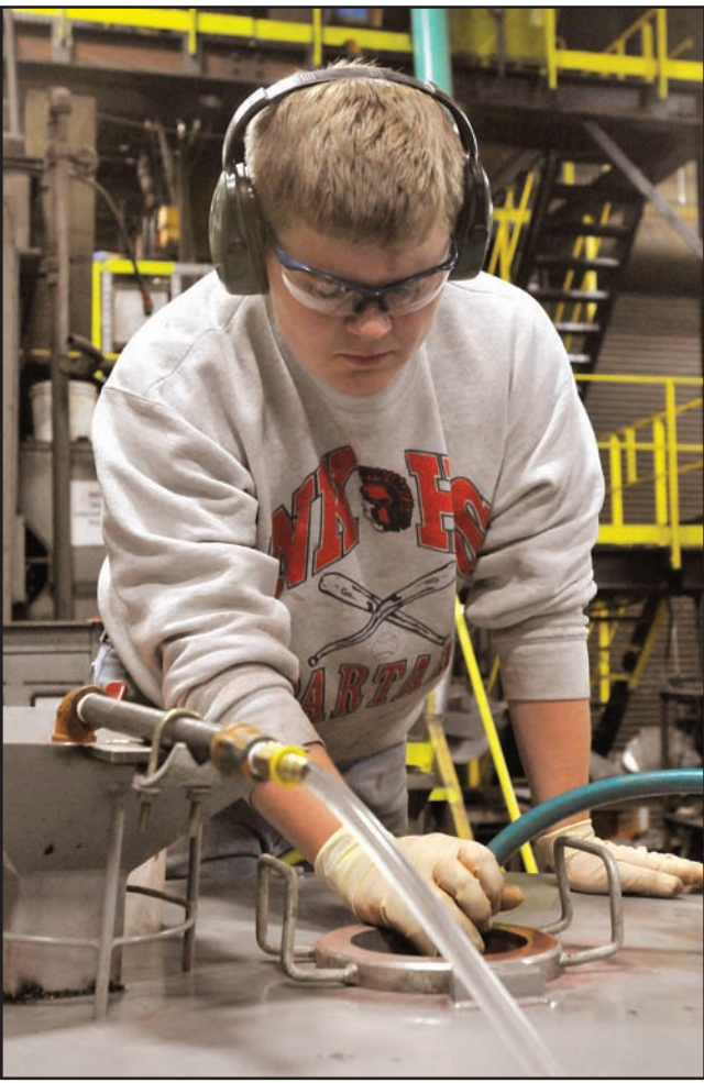
David Haugen adds water to a wet high intensity magnetic separator.
