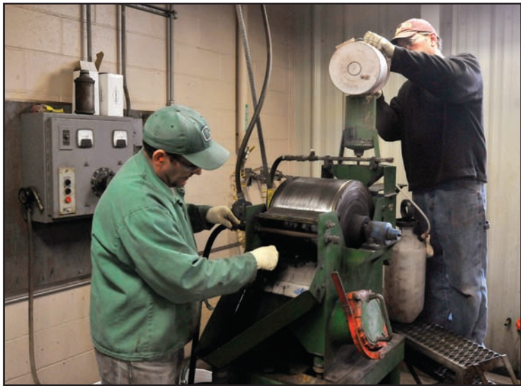
Shaun Gram and Donny Reiser pour a slurry of minerals through a low intensity magnetic separator at the Coleraine Minerals Research Lab.
