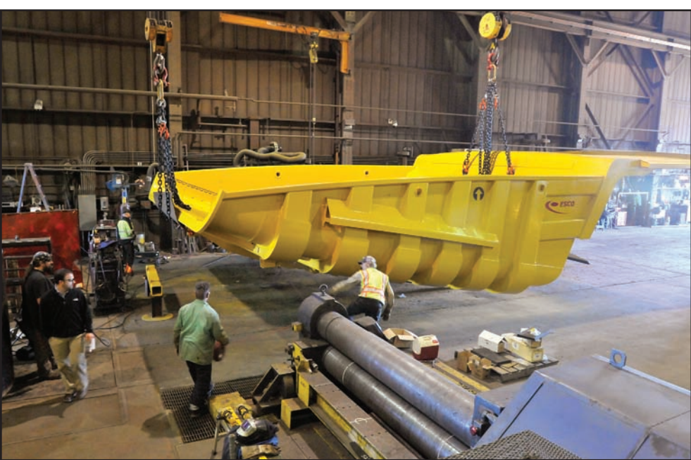
The first Esco truck bed manufactured at TRITEC is lifted between a pair of cranes.
