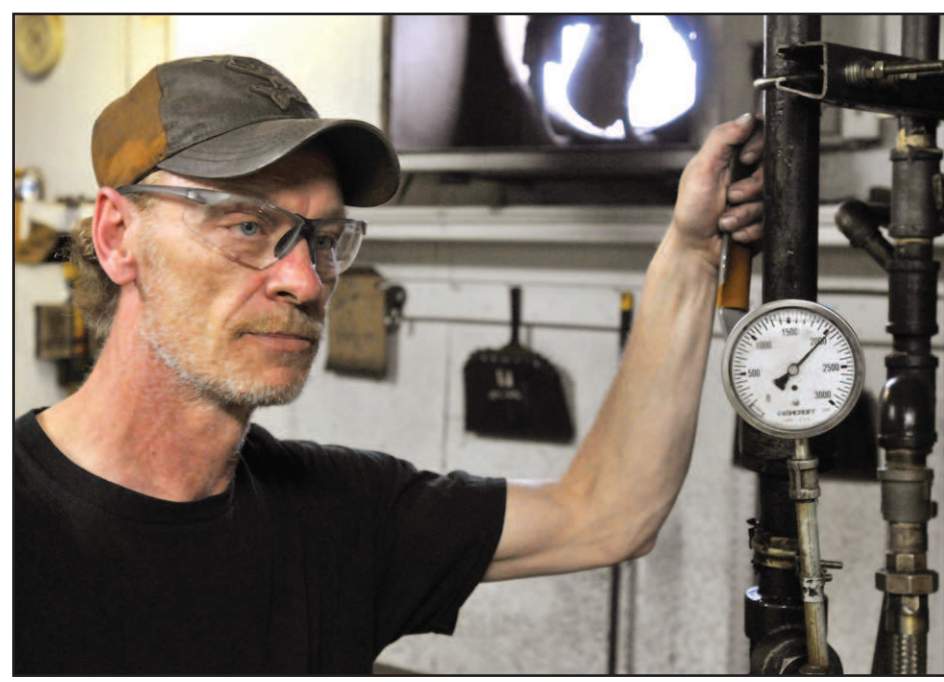
Carlson sets the press pressure to 2,000 psi to make an EZ Skirt product.
