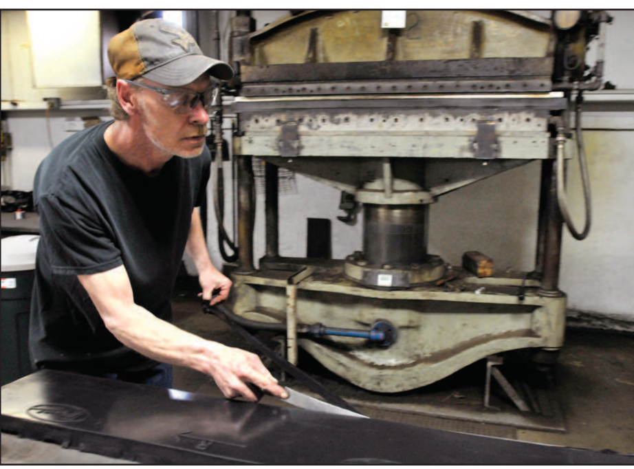
Kevin Carlson trims extra rubber from an EZ Skirt conveyor belt guard.
