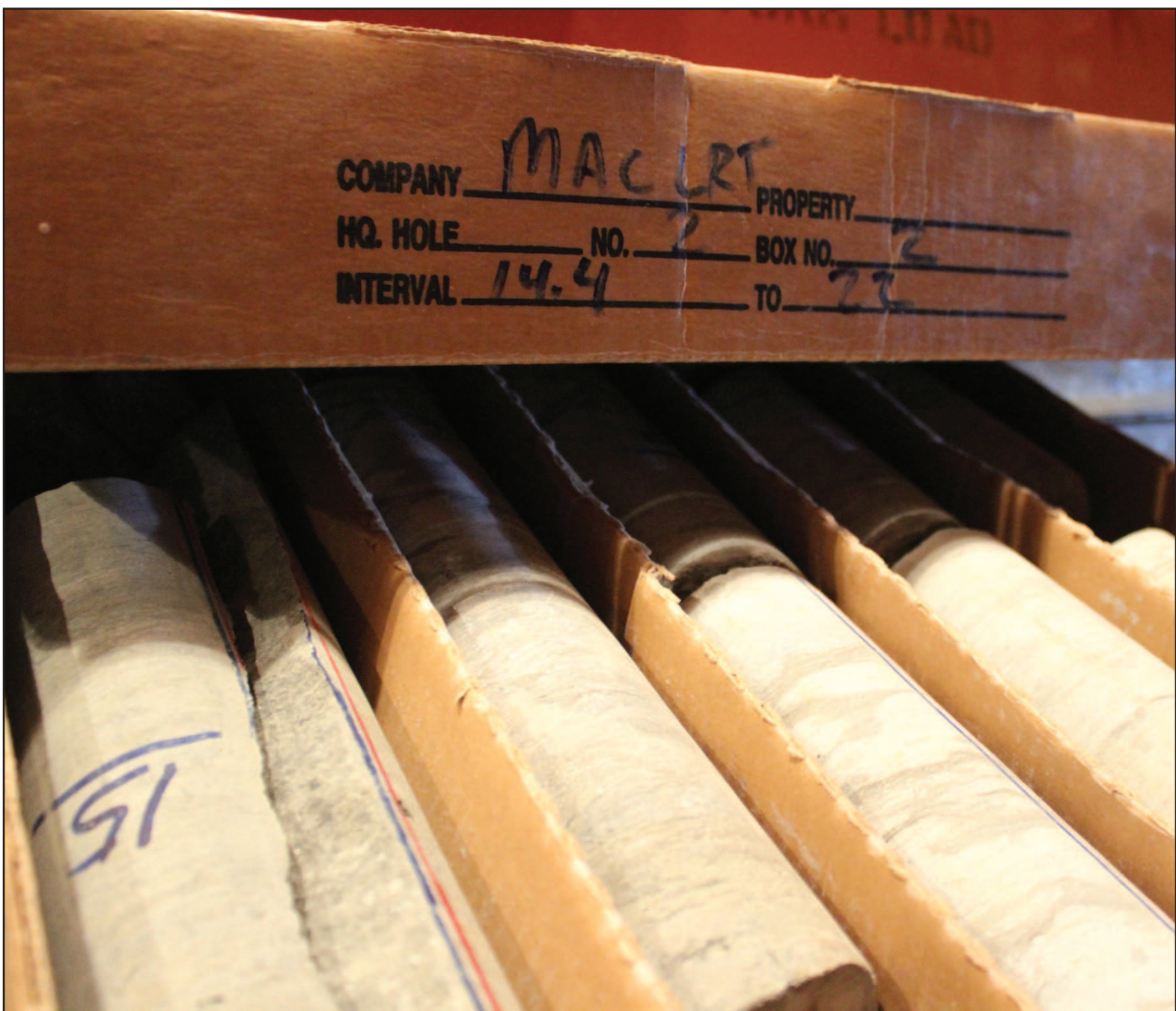
SEE LIBRARY, PAGE 23 A box containing core from the tunnel at the Minneapolis Lightrail is housed at the Core Drill Library.
