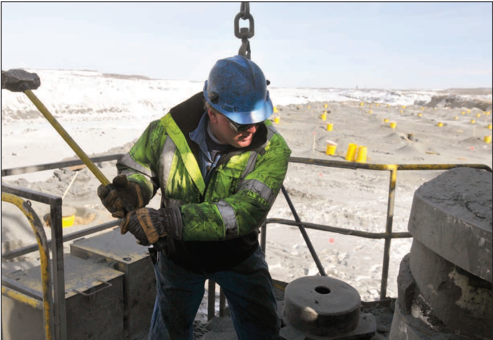
Jamey Sundberg uses a sledge hammer to knock into place a frozen coupling ring in a drill at Northshore in Babbitt.
