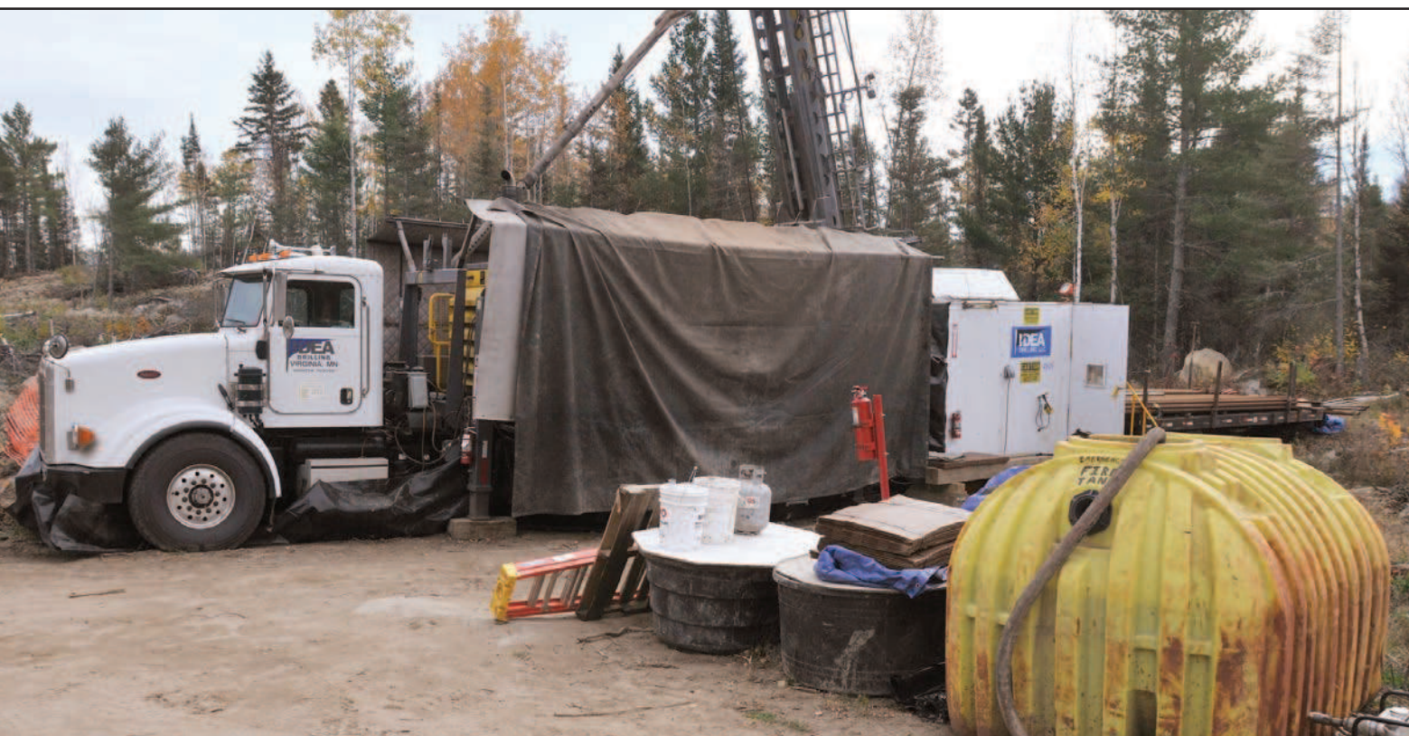
An IDEA Drilling crew works on a core sample at a test site near Ely. Crews have cut more than 500 test holes in the area looking for nonferrous metals.
