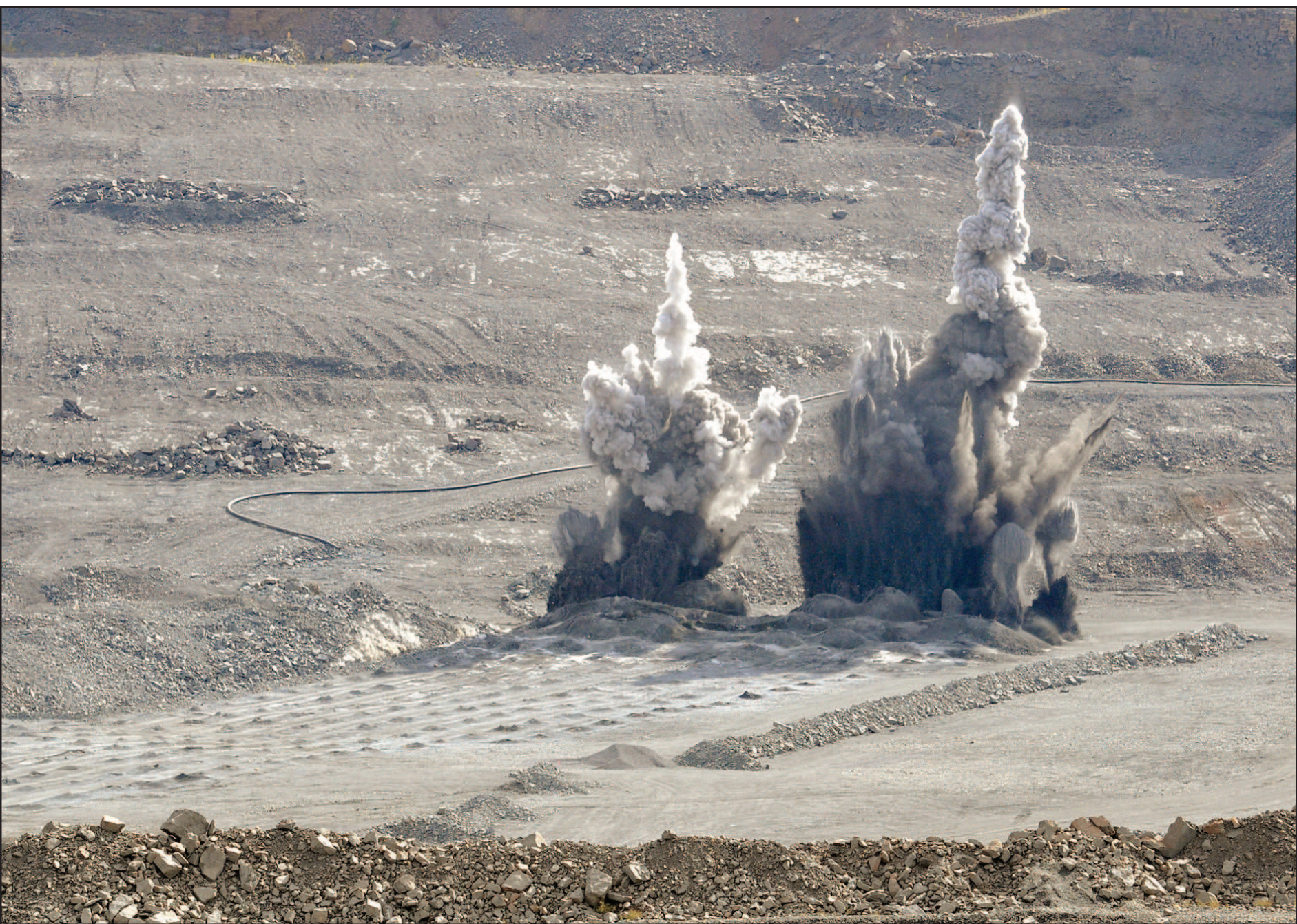
The blast begins on the far edge of the drill pattern.
