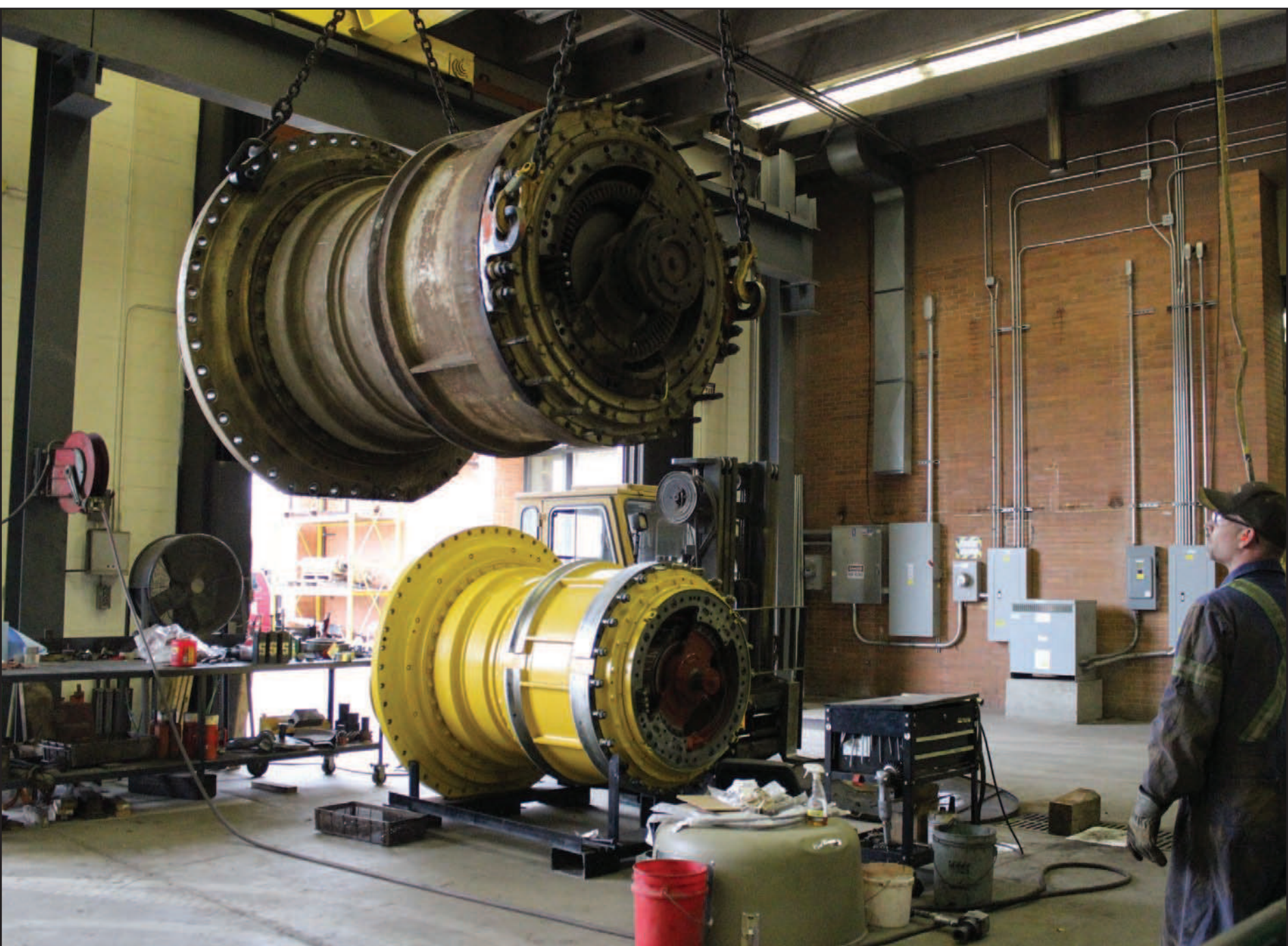
Josh Huhta carefully watches as a wheel motor for a 240-ton haul truck is moved by crane in Dom-Ex LLC's rebuild and service center located in Lees Central Business Center in Hibbing.
