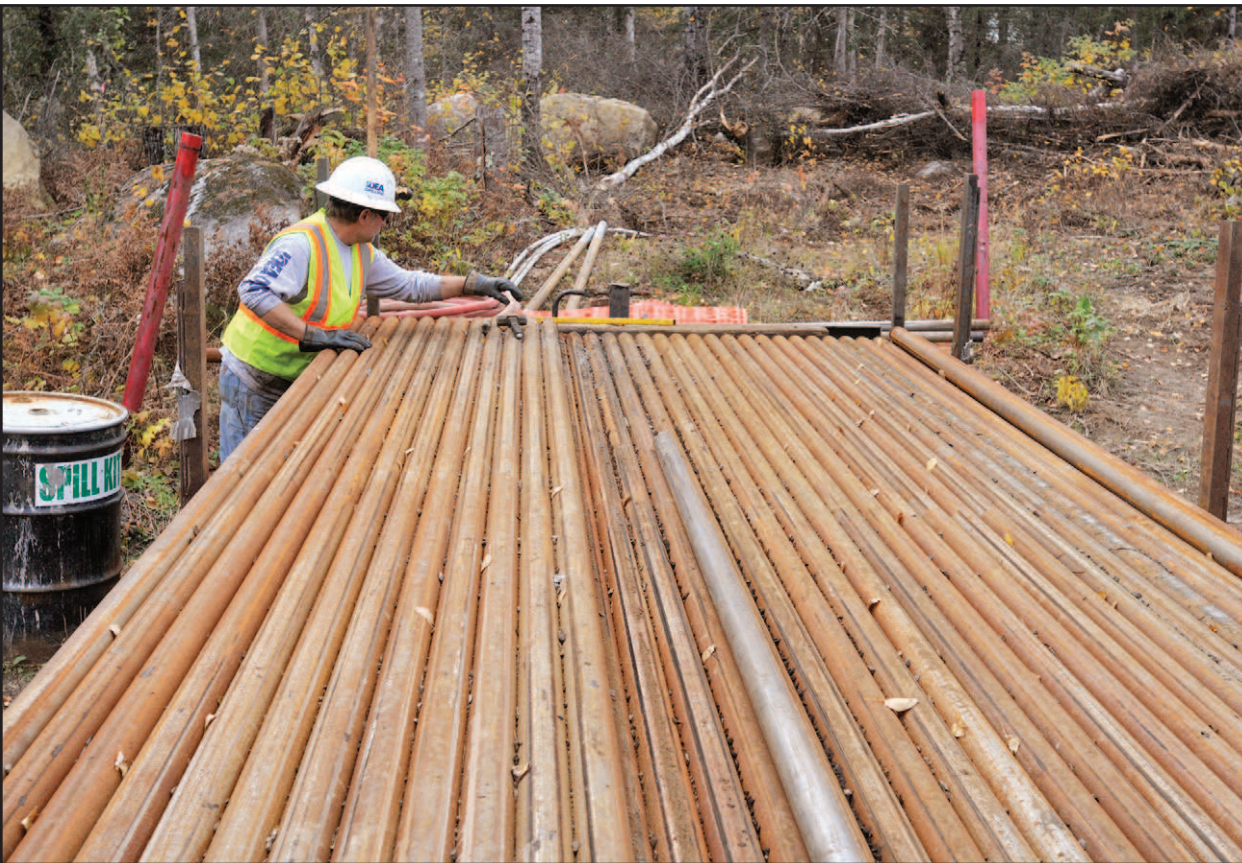
Bruce Ziminske checks drill pipe on a work site near Ely. The drill is capable of going more than 8,000 feet deep but most test holes are between 3,000 and 4,000 feet.
