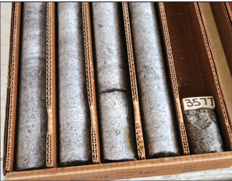
Core samples from 3,577 feet are marked and placed in a box for geologists to inspect.
