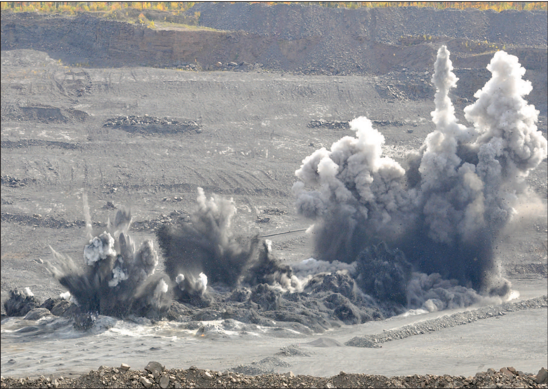
The blast continues to walk through the hole pattern. The whole sequence takes about five seconds.
