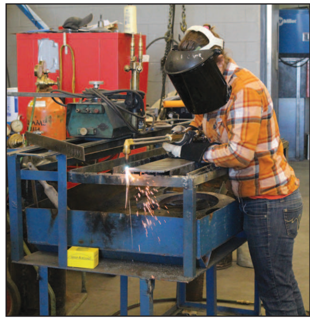
TONY POTTER/HIBBING DAILY TRIBUNE Lisa Alton, student of Industrial Systems Technology, uses an oxyacetylene torch to cut welding materials at Hibbing Community College
