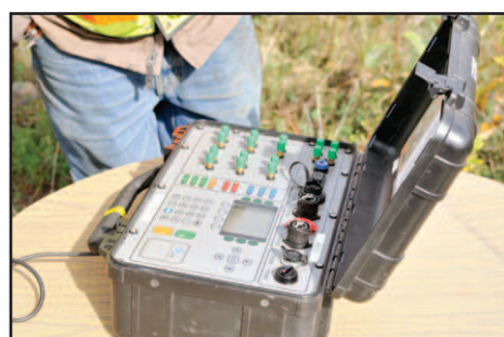
The electronic detonation system uses a two-key and two-button trigger, which makes an accidental blast impossible.
