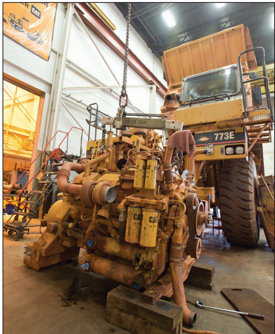
An engine is removed from a truck to facilitate repair.
